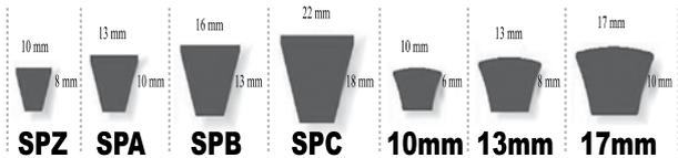
Narrow and classical sizes in molded notch construction. Lengths over 3,000mm are banded construction.
